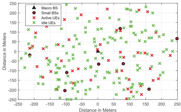
Fig. 5: Layout of the Simulated Heterogeneous Network
