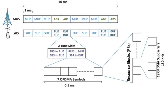
Fig. 2: Downlink Frame Structure
