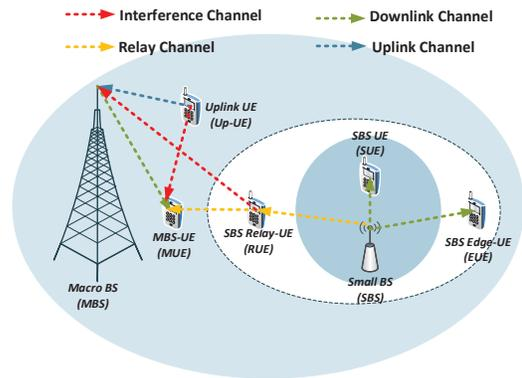
Fig. 1: Heterogeneous Radio Access Network System Model with Cell Range Expansion and Supporting D2D Communication
